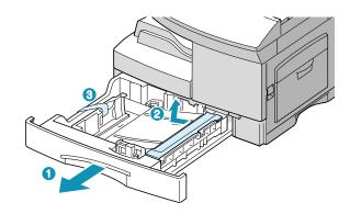
2 Push down on the pressure plate until it locks in position.
